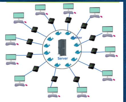
Powerful Server has been installed with all the necessary software's and Thin-Clients typically connects to this server through Remote Desktop connection over LAN.
